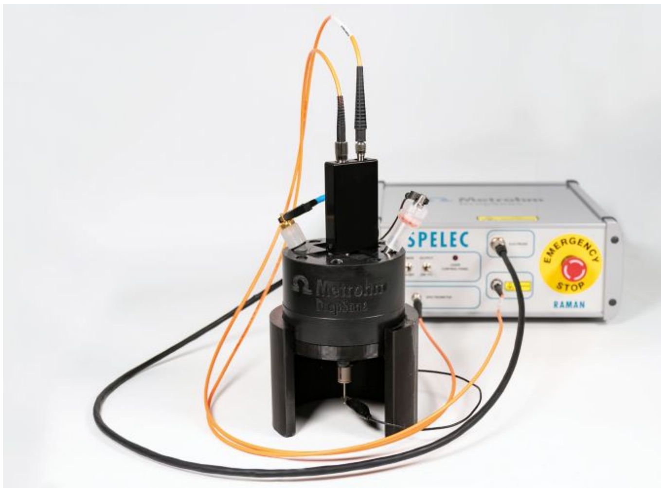
Figure 1. SPELEC RAMAN instrument and Raman probe used in combination with a Raman spectroelectrochemical cell for conventional electrodes.
