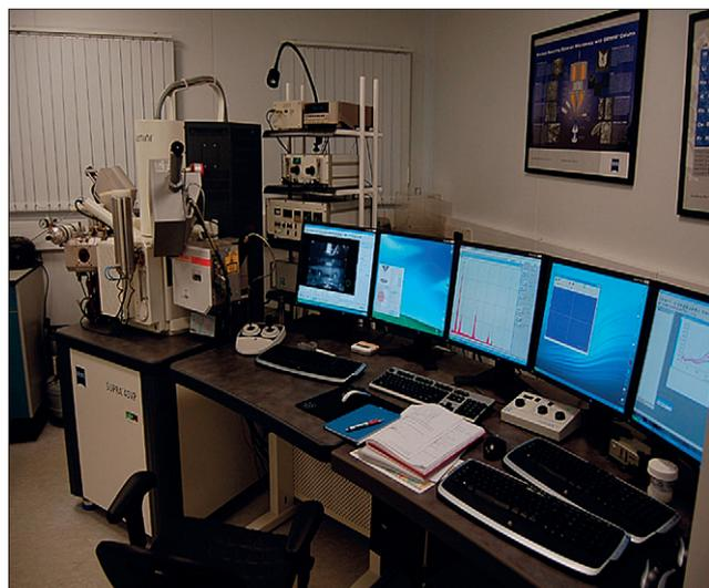
Figure 1. SEM/EDX interfaced with  $\mu$ RS (Renishaw SEM-SCA).
