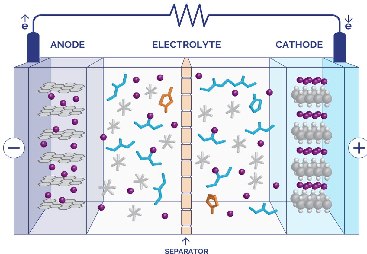
Figure 1: Diagram of a lithium-ion battery, showing major components including the anode, cathode, separator, and electrolyte.
