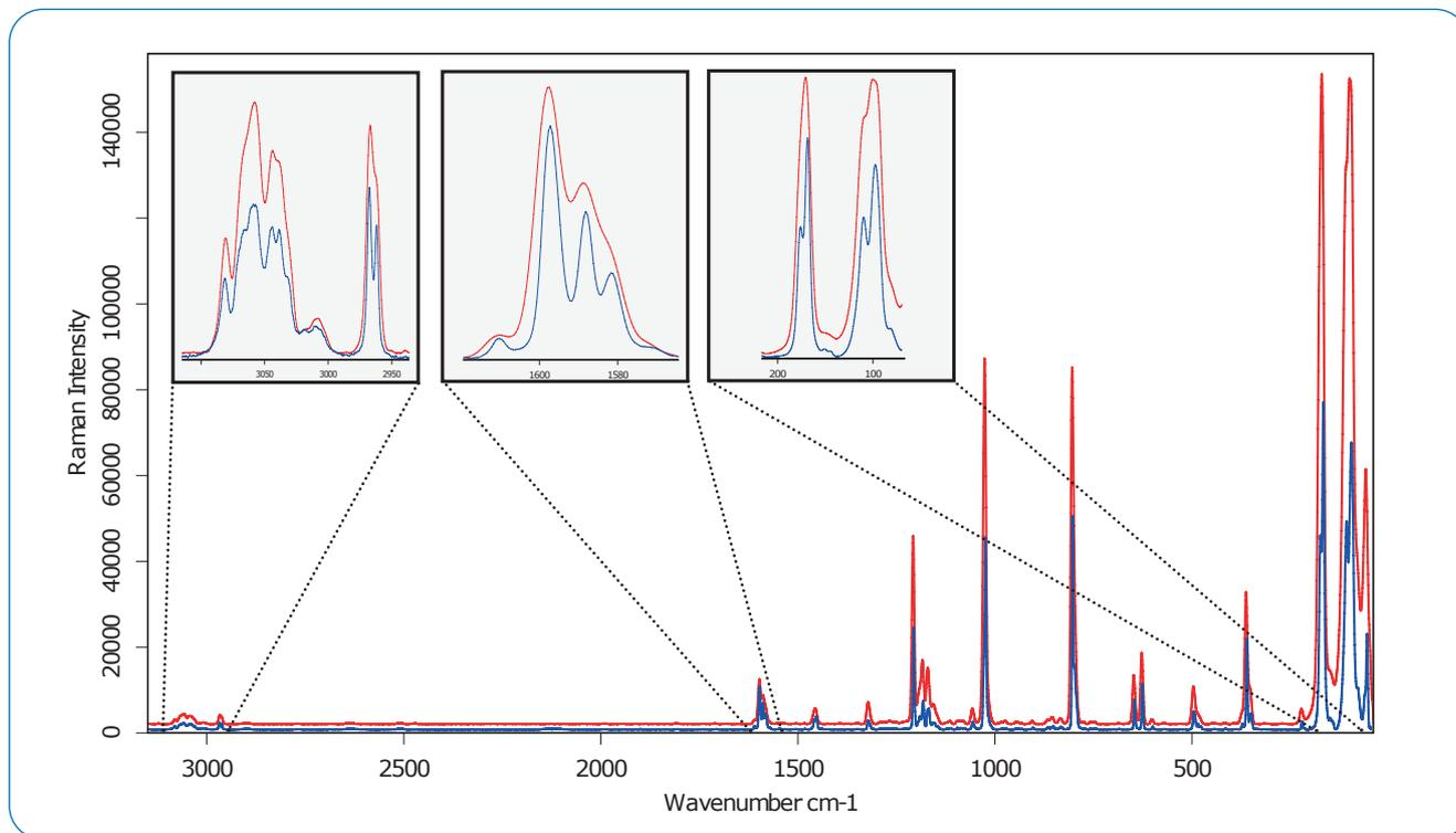
Figure 2: Raman spectrum of trypticene collected with full spectral range with the standard grating (4 cm<sup>-1</sup>, red) and the high-resolution grating (1.5 cm<sup>-1</sup>, blue). The highlighted areas show the obvious differences between the spectra.
