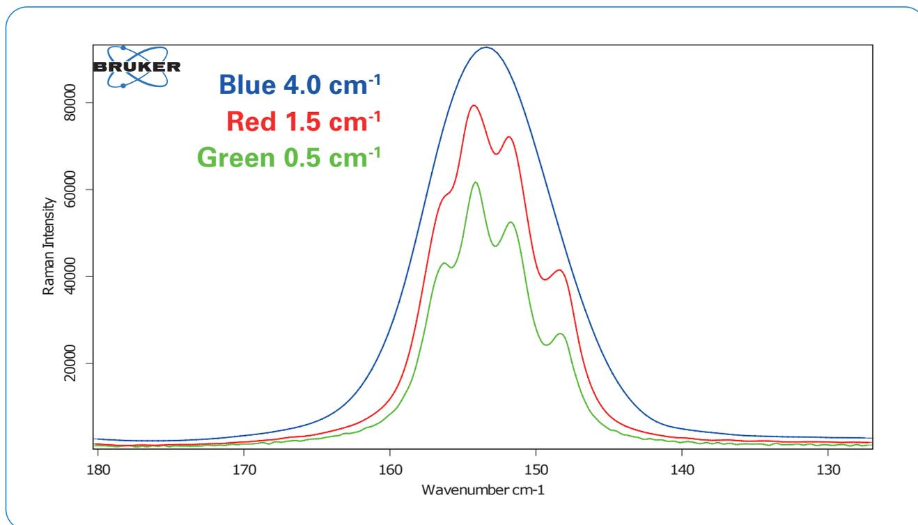
Figure 3: The Raman line of Sulfur at  $153\text{ cm}^{-1}$  acquired at different spectral resolutions with different instruments: Blue:  $4.0\text{ cm}^{-1}$  by SENTERRA II, 532 nm, grating: 400 gr/mm; Red:  $1.5\text{ cm}^{-1}$  by SENTERRA II, 532 nm, grating 1200 gr/mm; Green:  $0.5\text{ cm}^{-1}$  by MultiRam FT-Raman, 1064 nm.
