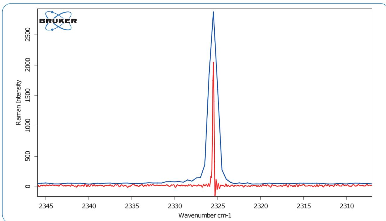
Figure 1: Raman spectra of the N-N stretching vibration of liquid nitrogen recorded with the dispersive Raman microscope SENTERRA II (blue spectrum, laser 785 nm) and the VERTEX/RAM II FT-Raman instrument (red spectrum, laser 1064 nm).
