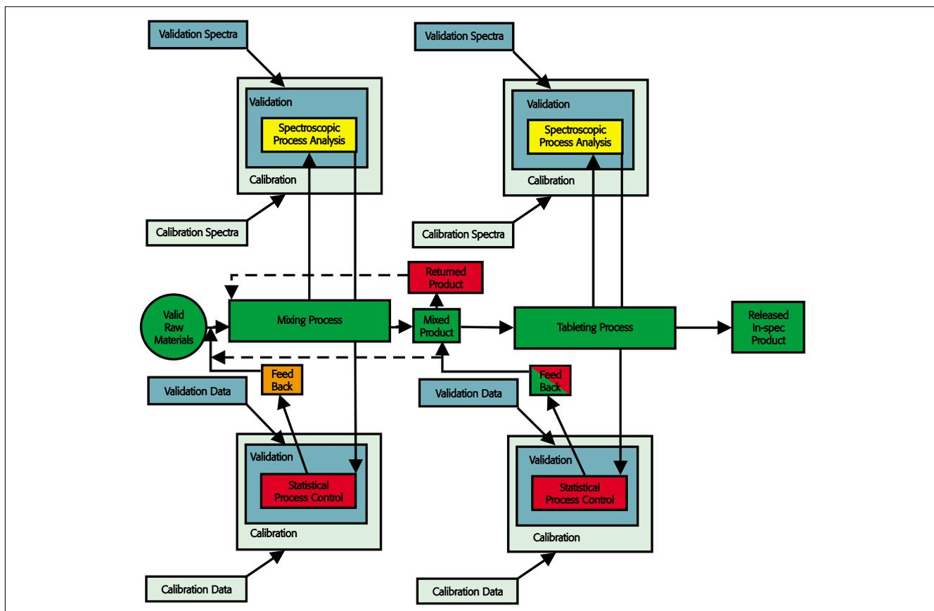
**Figure 3.** An outline of some of the chemometric operations required for a PAT two-stage process of mixing ingredients and forming the mixture into tablets.
