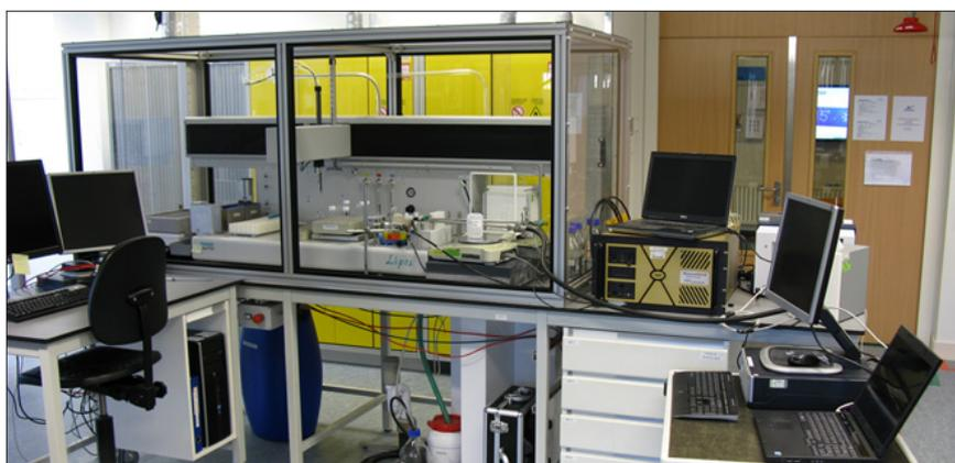
**Figure 3.** Zinsser robot at the Expert Capability Center in Deventer with integrated automatic spectroscopic analysis of the liquid samples created by the other high-throughput liquid handling robot.
