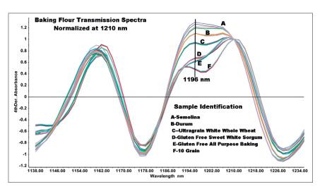
Figure 13. Fourth derivative spectra of the bread making flours after normalising at 1210 nm.
