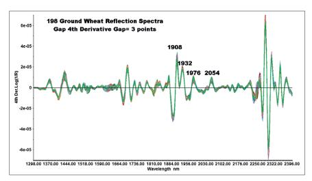
Figure 5. Fourth derivative spectra with a gap of three points for the 198 reflection spectra of wheat.
