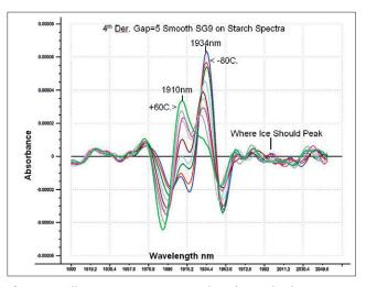
**Figure 2.** Diffuse transmission spectra of starch sample after conversion to the fourth derivative with a gap of five points.
