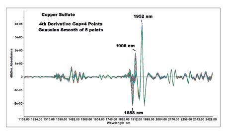
Figure 9. Fourth derivative spectra with a gap of four points for the copper sulfate samples.
