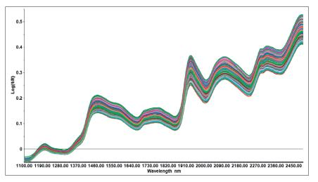
Figure 4. Diffuse reflection spectra of 198 ground wheat samples.
