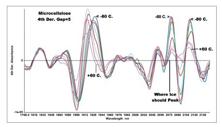
**Figure 3.** Diffuse transmission spectra of the microcellulose sample after conversion to the fourth derivative with a gap of five points.
