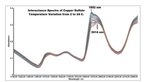
Figure 8. Interactance spectra of a copper sulfate sample at temperature range of 2°C to 24°C.
