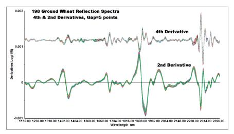
**Figure 6.** Second derivative and fourth derivative spectra with a gap of three points on the same 198 wheat samples.
