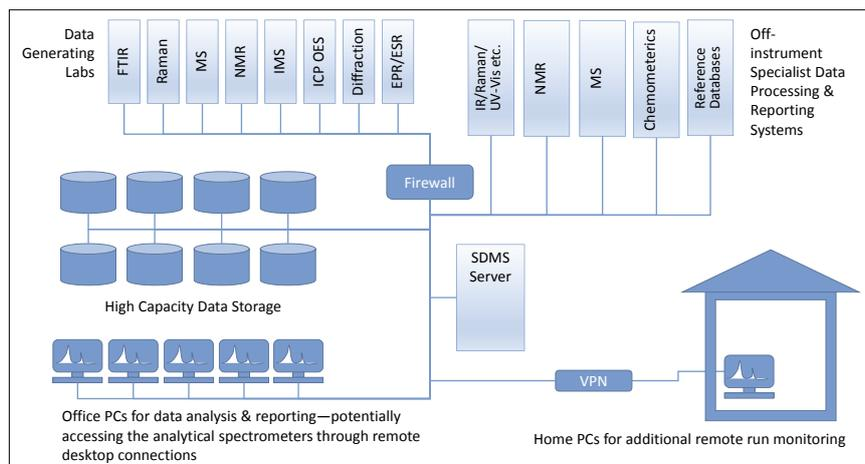
**Figure 2.** Potential for a Spectroscopic Data System—still a bit of a mess!
