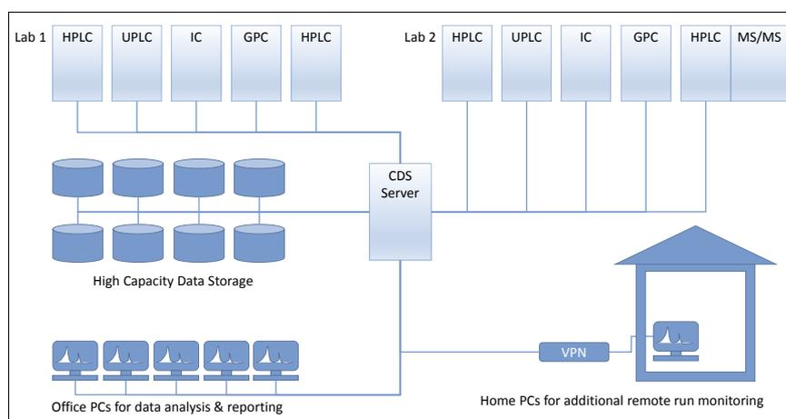
**Figure 1.** Potential modern CDS Deployment—now available with integrated mass spectrometry instrument control, data acquisition and analysis.
