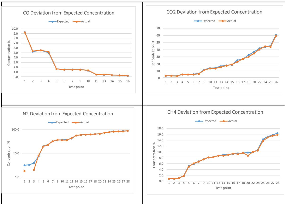
**Figure 2: Comparison of composition for CO, CO<sub>2</sub>, N<sub>2</sub>, CH<sub>4</sub> for syngas components**
