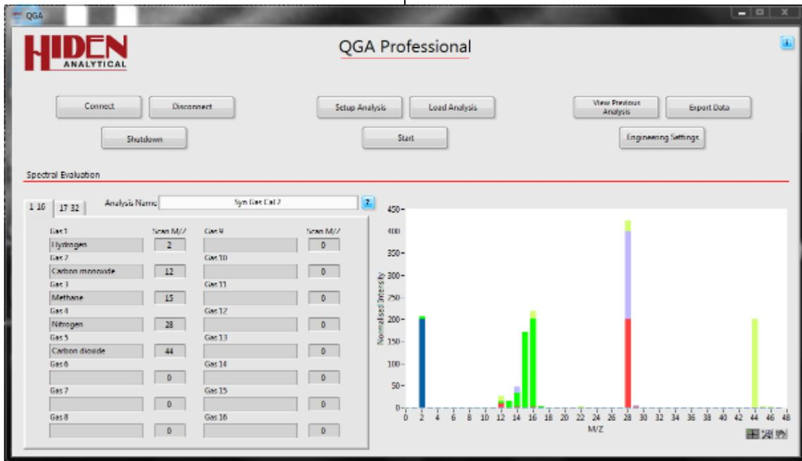
**Figure 1: QGA Professional screenshot showing gas components cracking pattern for syngas mixture**
