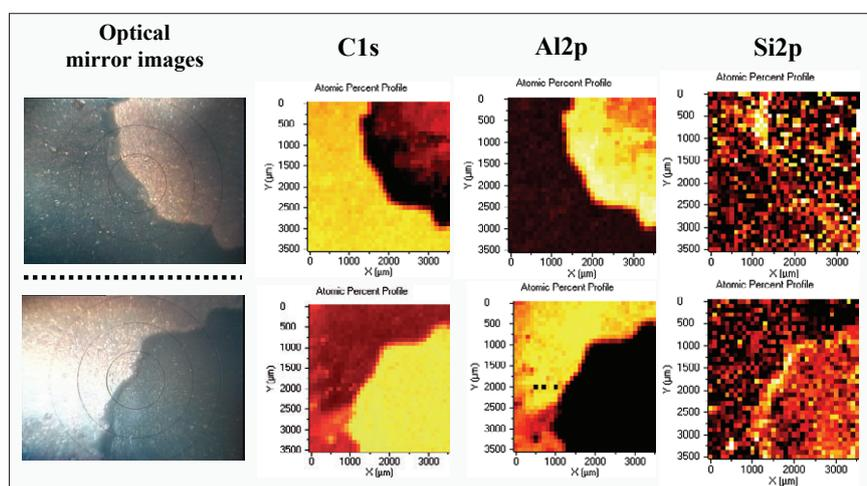
**Figure 2.** XPS images of the fracture surfaces taken from adhesively bonded aluminium using a structural epoxy adhesive with an addition of 1% organosilane adhesion promoter. (Courtesy of Dr M.-L. Abel, University of Surrey.)
