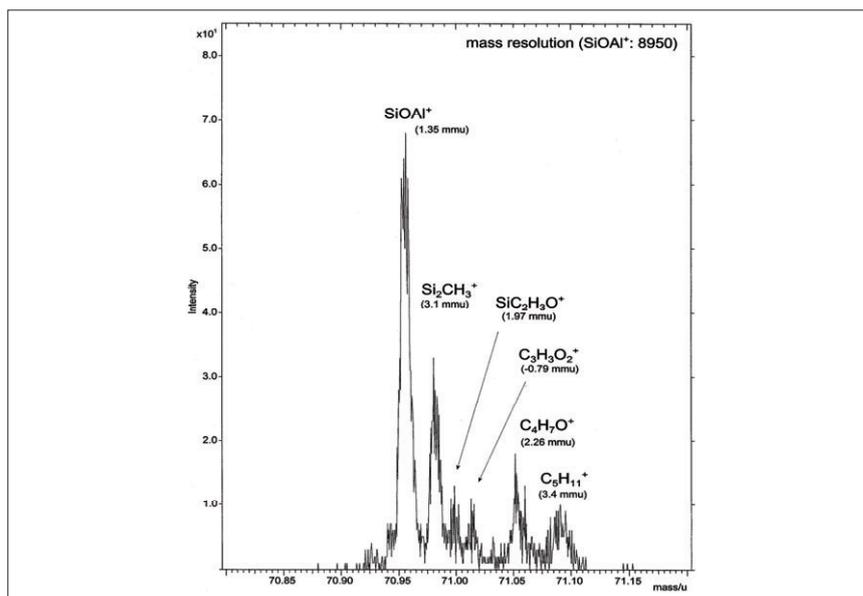
**Figure 4.** High-resolution positive ToF-SIMS spectrum of aluminium treated with an organosilane adhesion promoter. N.B. Total width of spectrum is c. 0.3u.
