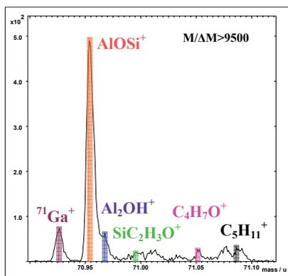
**Figure 5.** Positive ToF-SIMS spectra taken from the metal failure surface of adhesively bonded aluminium. The epoxy adhesive used contained 0.5% APS in the formulation. (Courtesy of Dr M.-L. Abel, University of Surrey.)
