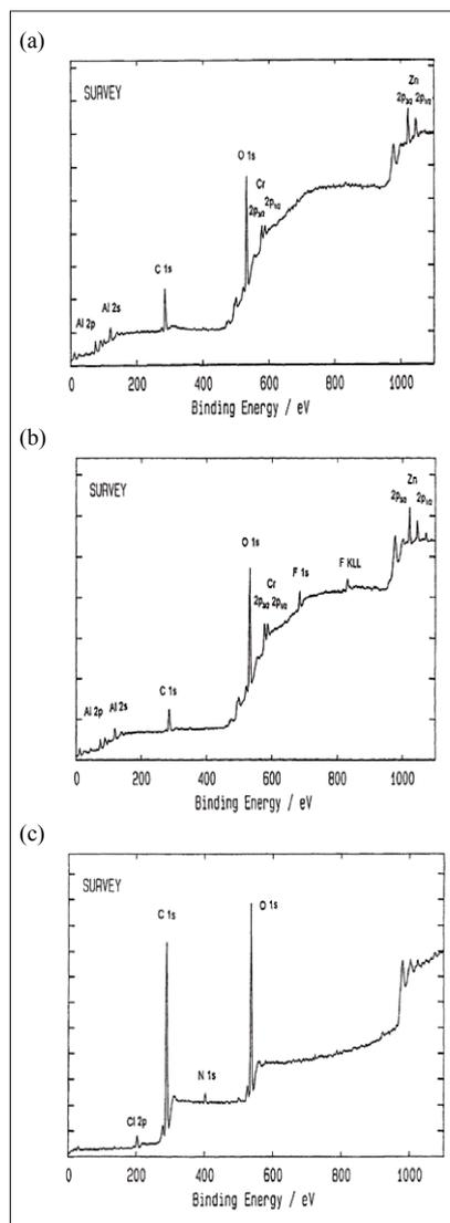
**Figure 3.** The failure of a radcure coating applied to galvanised steel. (a) uncoated steel, (b) steel interfacial failure surface, (c) coating interfacial failure surface.
