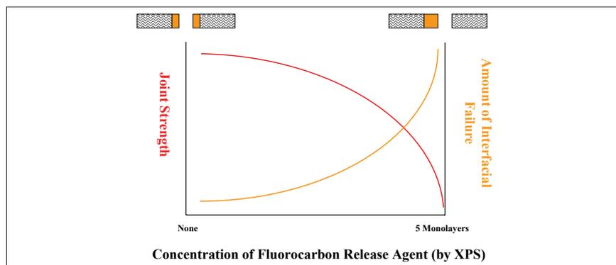
**Figure 1.** Correlation between residual release agent on a composite bonding surface and joint strength (LHS axis). As the strength reduces so the locus of failure changes from a cohesive failure in the adhesive (RHS axis and upper left schematic) to an interfacial failure between composite and adhesive (upper right schematic).
