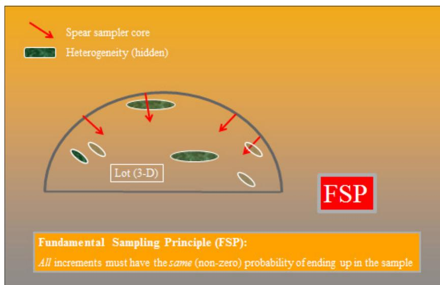
**Figure 5.** TOS' Fundamental Sampling Principle (FSP): "All virtual increments must have an identical, non-zero, probability to be extracted". Superficial spear sampling (never penetrating to the inner parts of the lot—red arrows) comprises a severe violation of FSP.
