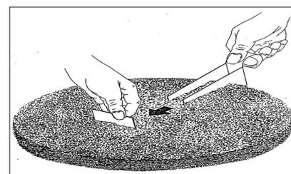
**Figure 2.** Severe over-sampling of the central parts of the lot; compare illustration above.
