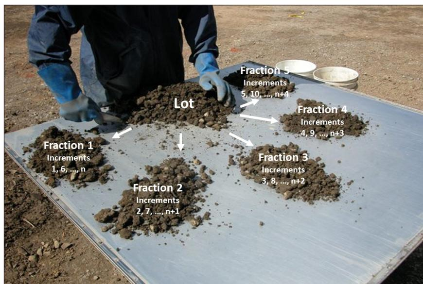
**Figure 2.** Primary samples obtained from the piles shown in Figure 1, which were reduced in the field using fractional shovelling as shown. Each fraction correspond to a final field sample sent to the laboratory. Secondary sample mass thus obtained was approximately 600 g of dry matter.
