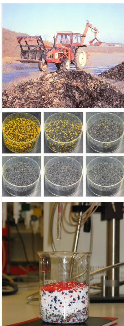
**Figure 3.** Compositional heterogeneity (CH) and distributional heterogeneity (DH) in real-world materials. How can one haphazardly selected “sample” (specimen) ever be assumed to be representative of an entire heterogeneous lot?
