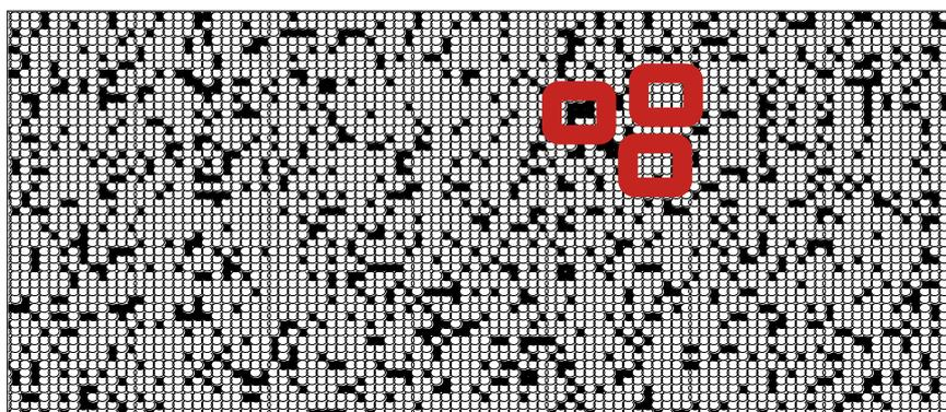
**Figure 4.** Any sampling process interacting with a material or a process stream that has the characteristics of significant distributional heterogeneity,  $DH_{lot}$  runs a fundamental risk of selecting and extracting worthless, non-representative **specimens**, a far cry from **representative samples**. The degree of risk is related both to the compositional as well as the distributional heterogeneity in relation to the sample mass employed.
