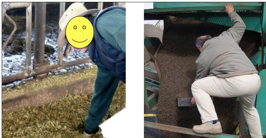
**Figure 2.** Two manifestations of simple grab sampling—as applied to significantly heterogeneous materials or processes.
