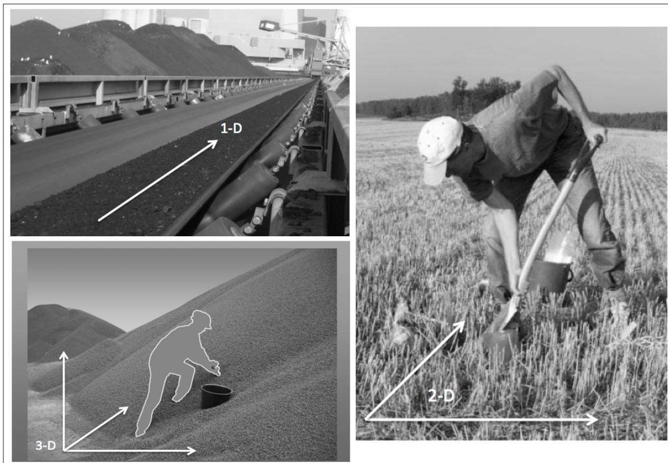
**Figure 2.** Lot dimensionality. Upper left: 1-D lot; right: 2-D lot; lower left: 3-D lot. TOS outlines that the principles behind representative sampling are scale-invariant (see text).
