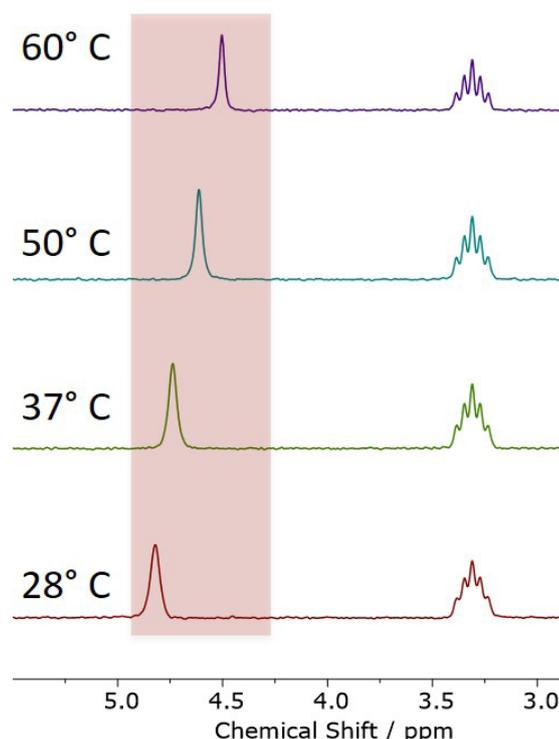
*MeOD-NMR Thermometer: MeOD spectra acquired at different temperatures. The chemical shift differences are in excellent agreement with the calibration values of the NMR thermometer.*
