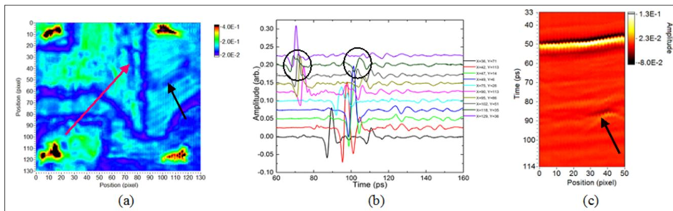
**Figure 3.** (a) Zone 5 peak-to-peak amplitude map of entire time-domain signal, (b) select time-domain waveforms and (c) a b-scan cross-section showing strong, possibly metallic, sub-surface feature in Zone 7.
