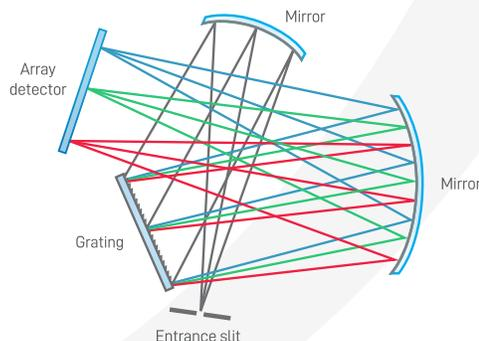
All-transmission spectrometer with VPH grating (left). Crossed Czerny-Turner spectrometer with reflective optics and ruled grating (right).
