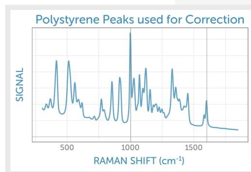
Example spectrum of glucose solution in a polystyrene cuvette. The polystyrene reference peaks are marked with vertical lines.
