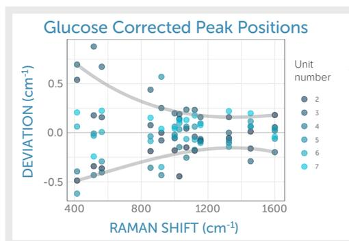
Deviation of glucose peak positions for individual spectrometers from the mean position across all spectrometers indicates a very narrow spread of less than 0.5 cm<sup>-1</sup> or less than 0.25 pixels.
