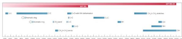
Figure 4: Raman functional groups by frequency, as compared to the operating range for a fingerprint (WP 785) and extended range (WP 785 ER) spectrometer
