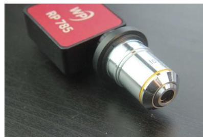
Figure 9: Wasatch Raman probe coupled with a microscope objective
