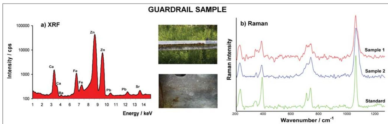
**Figure 1.** (a) XRF spectrum of the white spots of an old guardrail. (b) Raman spectra of the same spots on the guardrail together with the hydrozincite standard. The pictures in the middle were taken of a guardrail on the road and the piece of guardrail analysed in the laboratory on which the white spots can be seen.
