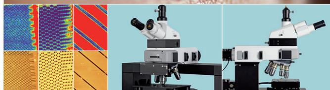
Raman stress and AFM topography images recorded automated at three different areas of a Si-device.
