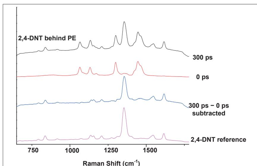
**Figure 2.** Explosives detection: TRRS of 2,4-DNT behind 5.0mm polyethylene (PE). The Raman spectrum at a short delay time (0 ps) that contains peaks exclusively of the first layer was scaled, then subtracted from the spectrum taken at a longer delay time (300 ps) that was composed of a mixture of first and second layer peaks. The result can be compared with a scaled reference spectrum of the second layer (2,4-DNT) at the bottom of the figure.
