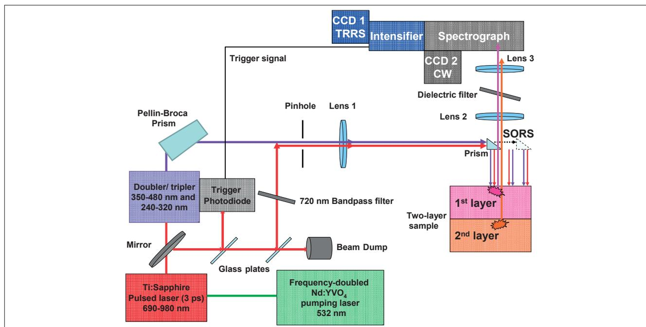
**Figure 1.** Instrumental setup for time-resolved Raman spectroscopy, spatially offset Raman spectroscopy or their combination (TR-SORS).
