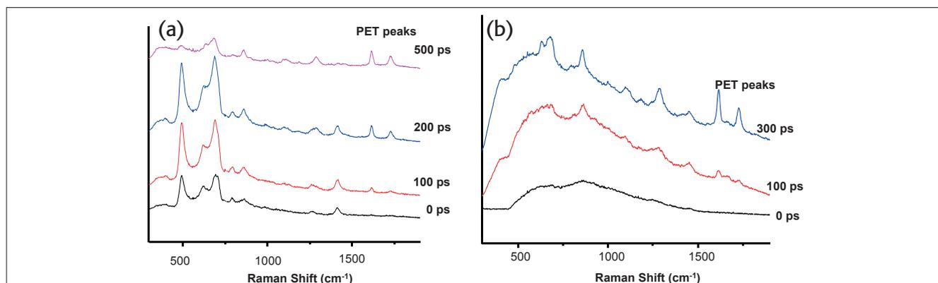
**Figure 3.** Through-skin measurements: TRRS depth profiling at different delay times of samples with (a) 2mm thick optical skin phantom of 0.4%  $\text{TiO}_2$  concentration or (b) 2mm thick porcine skin as first layer and PET as a second layer.
