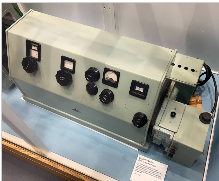
Figure 2. Pye Unicam SP500 UV/visible spectrophotometer. Photo © Ian Michael 2019, reproduced with kind permission of the Pye History Trust, Cambridge, UK.
