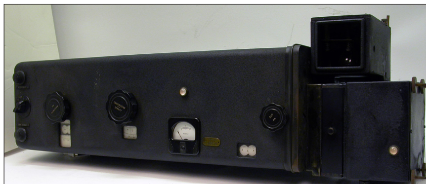
Figure 1. The Beckman DU spectrophotometer. Photo courtesy of the Beckman Institute for Advanced Science and Technology at the University of Illinois Urbana-Champaign
