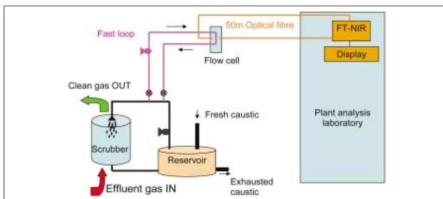
**Figure 1.** Diagram of caustic scrubber stream monitored by a remote FT-NIR analyser. In this example the system is an open loop (i.e. the analyser advises the operators of the caustic strength, but does not actuate valves itself), but would easily lend itself to full closed-loop control of the caustic strength.
