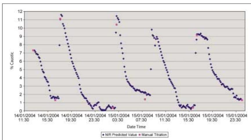
**Figure 5.** NIR monitoring of caustic scrubber strength (blue data). Note that only one NIR data point in five has been shown to aid clarity. NIR predictions were actually made every 100 s. The results of manual titrations are shown as purple data points. The diagram shows five cycles during which the scrubber is slowly exhausted and then recharged.
