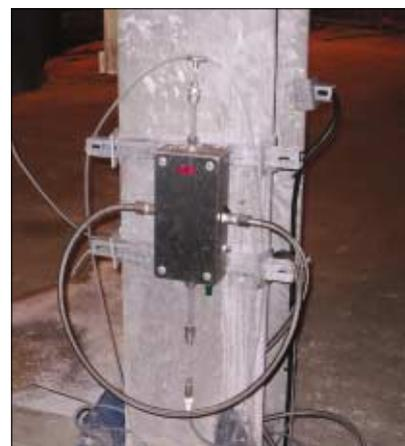
**Figure 2.** NIR flow cell installed in scrubber line at A.H. Marks. Caustic scrubber solution is pushed by a pump (bottom left) into the bottom of the cell and exits at the top. Fibre optic connections enter via the stainless steel conduits on each side of the cell.
