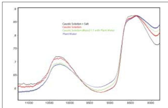
**Figure 4.** The blue, red and green NIR spectra are of plant water, caustic solution and diluted caustic solution, respectively. The addition of salt (NaCl), which has no NIR spectrum of its own, to the caustic solution (black spectrum) alters the OH signals of the caustic/water spectrum significantly. This effect can interfere with calibrations for caustic strength, particularly at low caustic concentrations.
