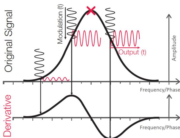
**Figure 5.** Top-of-fringe principle. Modulating the laser frequency and demodulating the PD signal with the same frequency leads to an error signal which is proportional to the derivative of the original signal.
