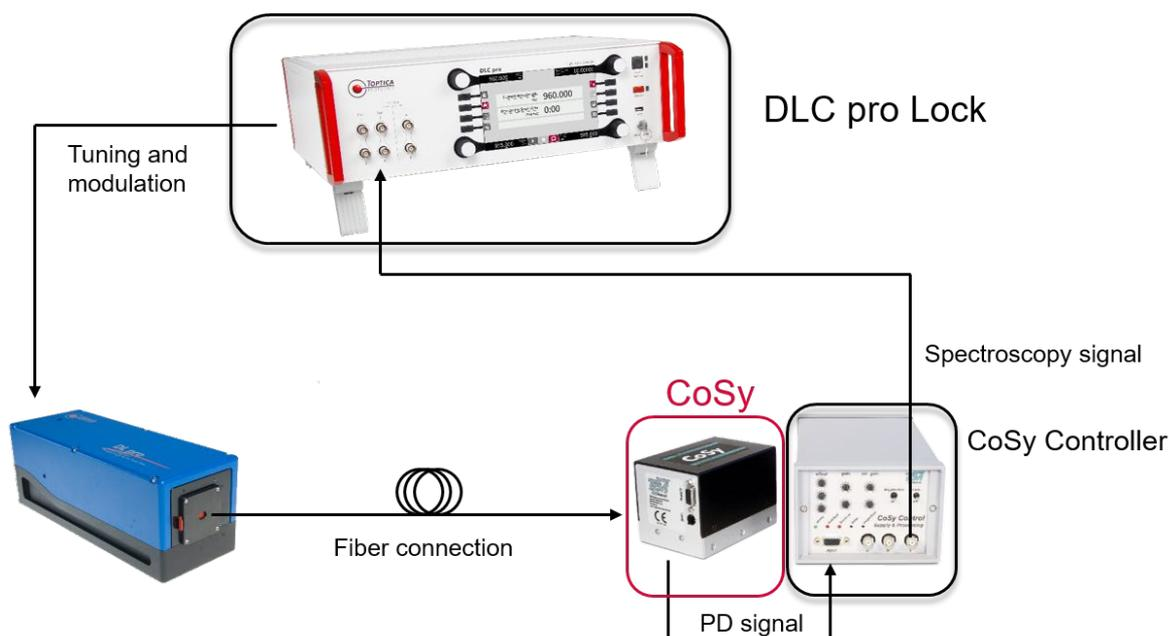
**Figure 9.** Schematic of a spectroscopy lock using TOPTICA components.
