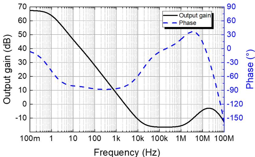
**Figure 15.** Example of a transfer function as obtained with TOPTICA’s fast PID regulator FALC 110. The amplitude of the transfer function (black) describes the frequency-dependent gain of the controller. The phase of the transfer function (blue) describes the phase difference between the input and the output signal.
