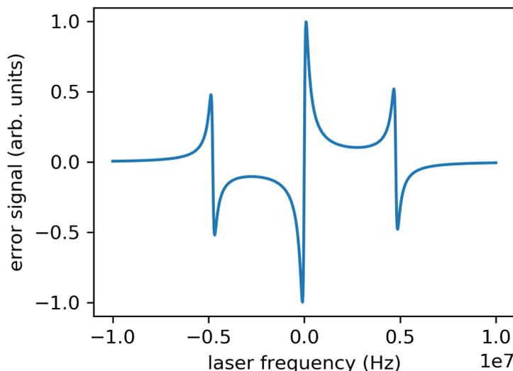
**Figure 12.** PDH error signal. It features a steep slope around the lock point at 0 Hz and a large capture range determined by the modulation frequency of 5 MHz. The second and third zero crossing at -5 and +5 MHz correspond to one sideband being resonant with the cavity and interfering with the reflected carrier and other sideband.
