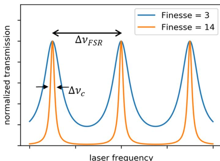
**Figure 10.** Transmission of a Fabry-Pérot resonator. High reflectivity of the mirrors (orange) leads to a small spectral width  $\Delta\nu_c$ . The distance between cavity resonances  $\Delta\nu_{FSR}$  is determined by the length of the resonator.
