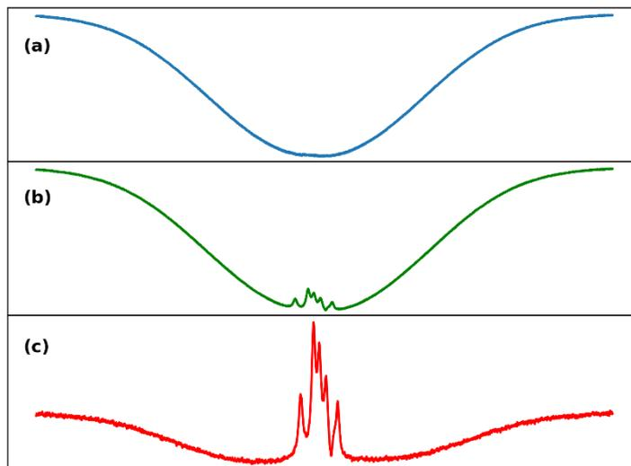
**Figure 7.** (a) Doppler-broadened spectrum; (b) Spectrum obtained from Doppler-free saturation spectroscopy; (c) Doppler-free spectrum reduced by Doppler broadened spectrum
