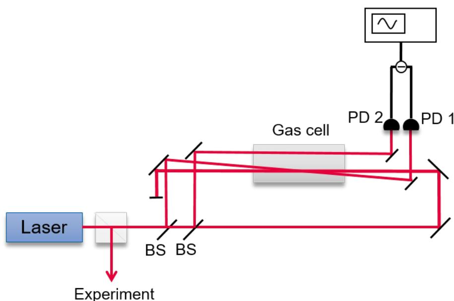
**Figure 6.** Optical setup for Doppler-free saturation spectroscopy. A strong pump beam is counter-propagating the weak probe beam. If the laser hits a resonance, pump and probe beam address the same group of atoms that have zero velocity along the beam axes. The strong pump beam saturates those atoms such that probe light absorption is minimal. This leads to high transmission of the probe beam.
