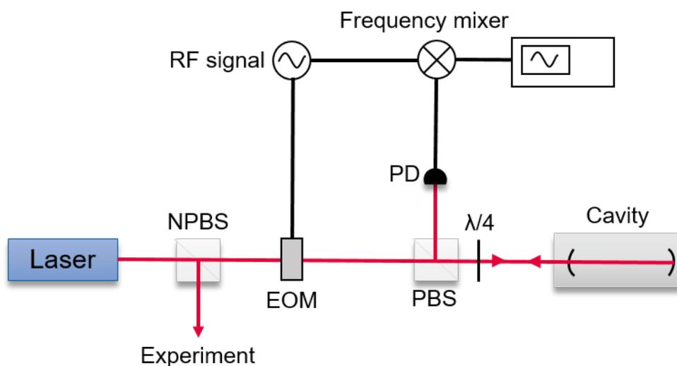
**Figure 11.** Schematic setup for the Pound-Drever-Hall technique. Optical paths are depicted in red, electronic signal paths in black.
