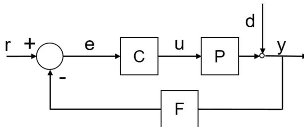
**Figure 14.** Diagram of a closed loop system. The reference signal  $r(t)$  is compared to the output signal  $y(t)$  which is measured with a sensor  $F$ . The difference between these signals is the error signal  $e(t)$  which is processed by the controller  $C$  and generates the control signal  $u(t)$ . The control signal is fed into the plant  $P$  which generates the output signal  $y(t)$ .  $d(t)$  describes noise which perturbs the system.
