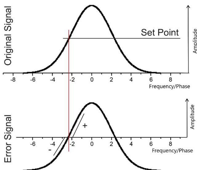
**Figure 4.** By adding or subtracting a constant value, an error signal can be obtained from a spectral peak or dip.
