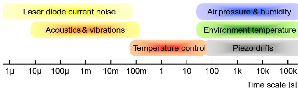
**Figure 2.** Sources of laser noise.
