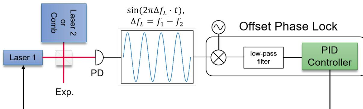
**Figure 13.** Optical setup for the implementation of an offset phase lock.
