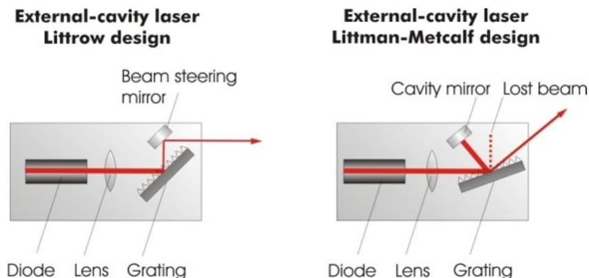
**Figure 16.** Different configurations of external cavity diode lasers (ECDL).
