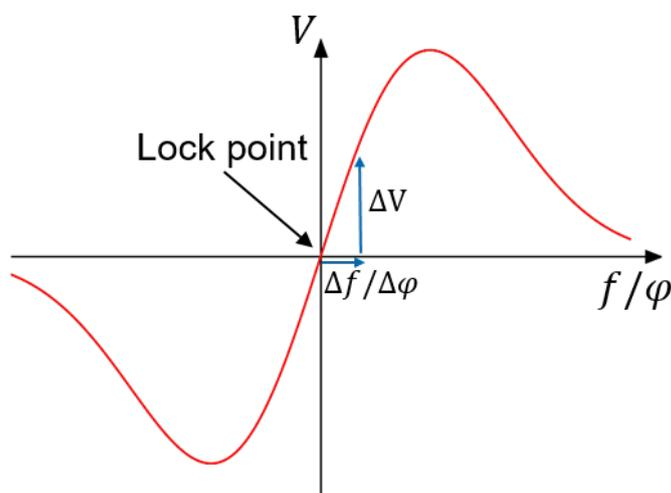
**Figure 3.** Sketch of a typical error signal. The lock point is given by the zero-crossing. The steepness of the slope around the zero-crossing affects the sensitivity of the signal to phase or frequency fluctuations. Ideally, the error signal would be a purely linear function of phase or frequency. However, the error signal shown here is more realistic as it is given by the derivative of a spectral peak or dip.
