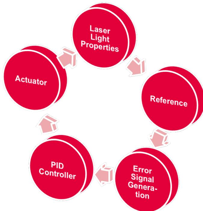
**Figure 1.** Diagrammatic concept of a feedback loop for phase and frequency locking.
