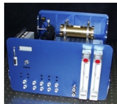
Figure 4. Photograph of the PASS (photoacoustic soot sensor) system.
