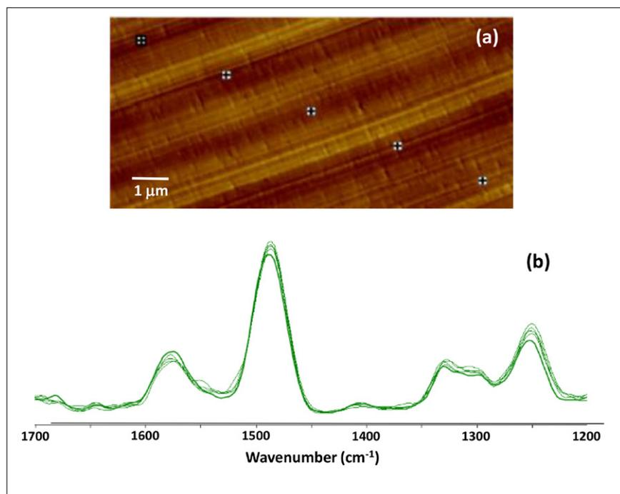
**Figure 6.** AFM topography (a) and AFM-IR spectra (b) of the same two polymer components as shown in Figures 4 and 5, but blended under different processing conditions. This time the mixing of the two components is more uniform.
