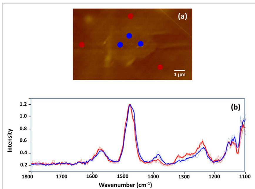
**Figure 5.** AFM topography (a) and AFM-IR spectra (b) of the same two polymer components shown in Figure 4, but blended under different processing conditions. The region at the centre of the image where the blue AFM-IR spectra were collected show a different level of mixing of the two components compared to the surrounding region where the red spectra were collected.
