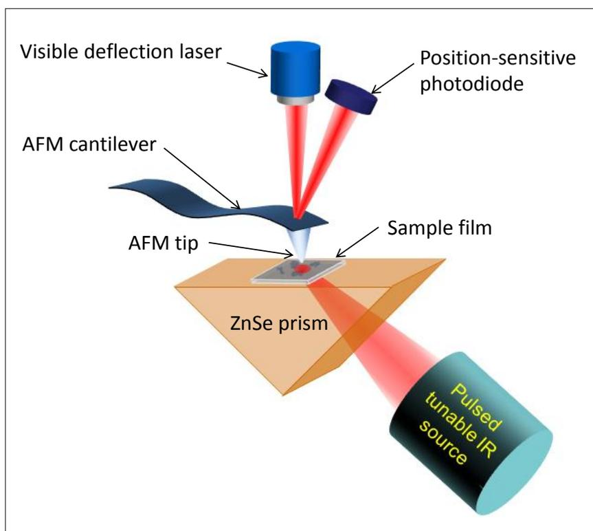
**Figure 1.** The AFM-IR technique uses a pulsed, tuneable IR source to excite molecular vibrations in the sample. Absorption of IR radiation by the sample leads to a rapid thermal expansion that excites resonant oscillations of the cantilever. The AFM cantilever ringdown amplitude plotted as a function of the laser wavenumber produces the IR spectrum.
