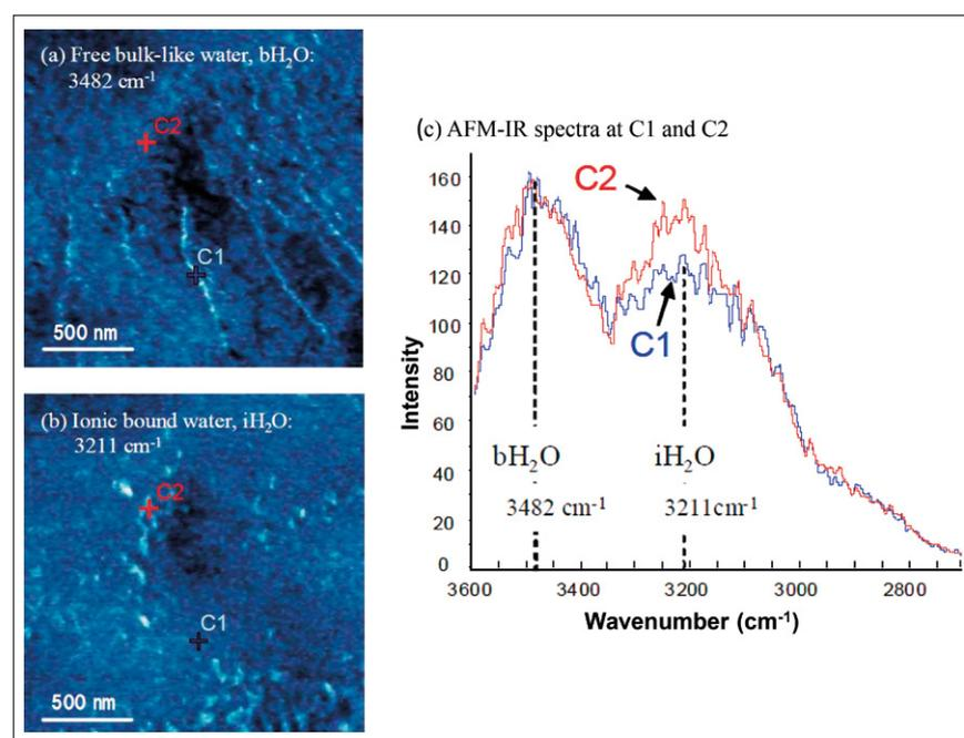
**Figure 2.** AFM-IR chemical images of water within a Nafion film: (a) bulk-like water at  $3482\text{ cm}^{-1}$ ; (b) ionically bound water at  $3211\text{ cm}^{-1}$ ; and (c) AFM-IR spectra at points C1 and C2. Image (a) and the spectra (b) show that bulk-like water and ionically bound water are distributed differently on the Nafion membrane surface.<sup>10</sup>
