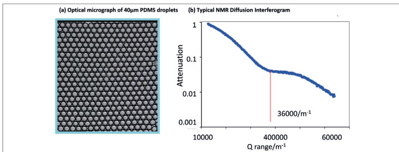
**Figure 3.** (a) Optical micrograph of 40  $\mu\text{m}$  PDMS droplets, (b) typical NMR Diffusion Interferogram.
