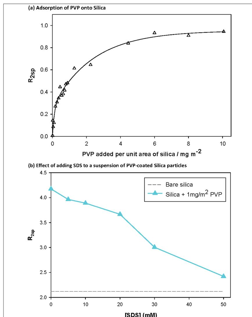
**Figure 2.** (a) Adsorption of PVP onto silica, (b) effect of adding SDS to a suspension of PVP-coated silica particles.
