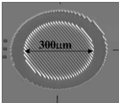
**Figure 2.** Micro-lens preform prior to mass transport.
