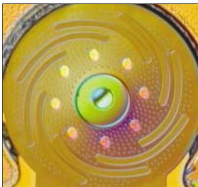
**Figure 6.** MEMS Tunable Fabry-Perot Mirror. This assembly is about 1 mm wide.
