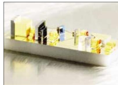
**Figure 1.** Micro-spectrometer components on aluminium nitride optical baseplate. The bench is 14 mm long.
