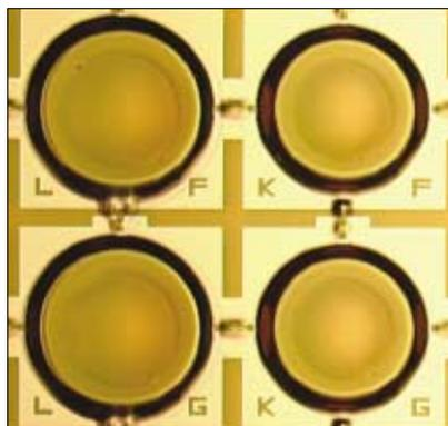
**Figure 3.** Mass transported micro-lenses prior to dicing showing mounting pads and alignment marks.
