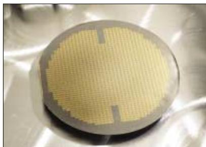
**Figure 5.** An array of Fabry-Perot tunable filter mirrors on a 4 inch silicon wafer.
