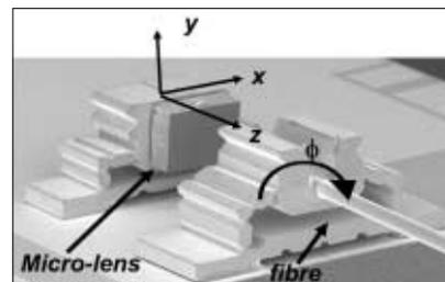
**Figure 4.** Scanning electron micrograph of two LIGA structures: holding a lens and a single-mode fibre optic, showing the degrees of freedom available in the alignment process.
