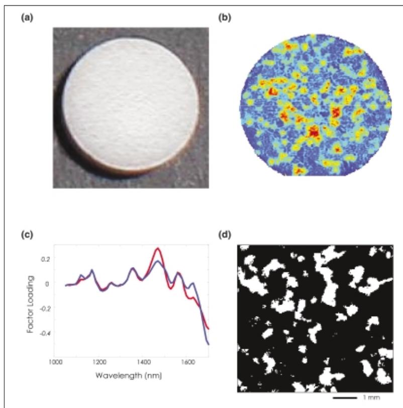
**Figure 2. (a) Visible image of an over-the-counter plain medication tablet. (b) PCA score plot for factor 3. (c) ALS “pure” component loading spectra for the API and Excipient mixture. (d) Concentration estimate image. White pixels represent the API with an estimated bulk concentration of 19.38%.**
