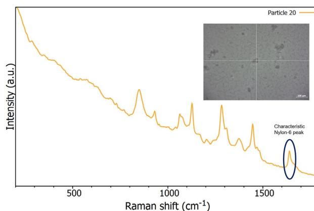
Figure 5: Spectra and white light image from particle 20
