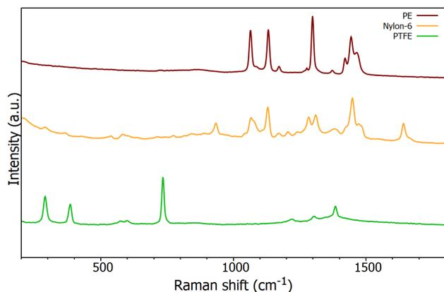
Figure 2: Raman spectra of nylon-6, PE, and PTFE
