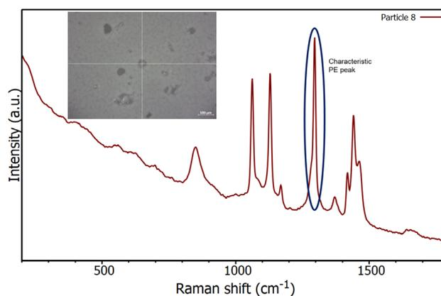
Figure 4: Spectra and white light image from particle 8
