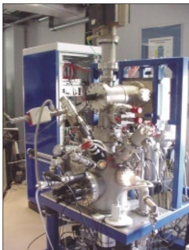
**Figure 3.** Photograph of the Cation Mass Spectrometer.
