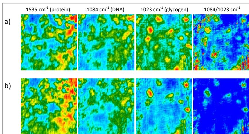
**Figure 3.** False-colour, macro ATR FT-IR images of the distribution of the integrated absorbance of the amide II, DNA and glycogen bands after (a) incubation overnight on the diamond crystal and (b) 90 min. Adapted from Reference 2 with permission from the Society for Applied Spectroscopy.
