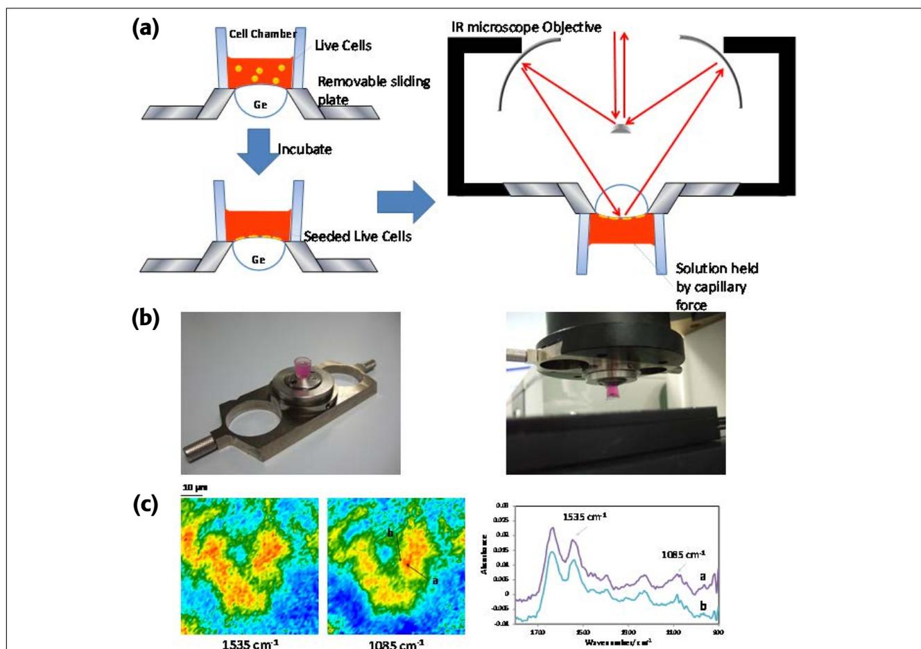
**Figure 2.** ATR FT-IR imaging of live cells in micro ATR mode. Cells were incubated directly onto a removable slide Ge ATR crystal and introduced into an IR microscope shown (a) schematically and (b) photographed. (c) The resulting false-colour images due to: left, amide II, and right, phosphate (nucleic acid) absorbance, as well as extracted spectra. Kazarian & Chan, *Analyst*, 1940 (2013)—Reproduced by permission of The Royal Society of Chemistry
