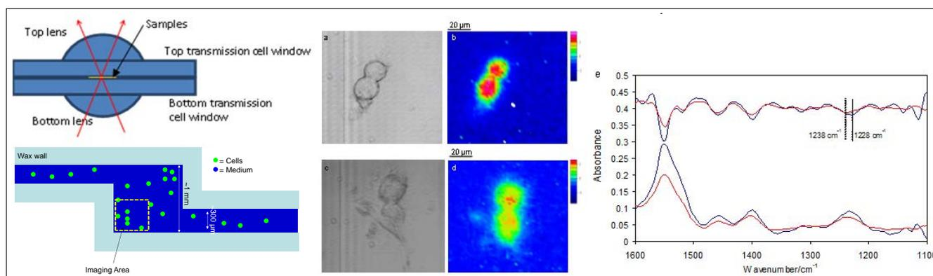
**Figure 4.** (a) Microfluidics-based transmission mode imaging of live cells with a pseudo-sphere to correct chromatic aberration shown schematically. (b) White light and amide II false-colour FT-IR images are shown before (upper) and after (lower) cell spreading and (c) extracted spectra (bottom) and derivatives (top) are plotted to show shift in phosphate (nucleic acid) band upon spreading. Chan & Kazarian, *Analyst* 4040 (2013)—Reproduced by permission of The Royal Society of Chemistry.
