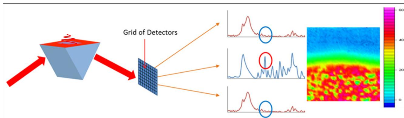
**Figure 1.** A schematic of ATR FT-IR imaging. IR light is incident on an ATR crystal above the critical angle. An evanescent wave penetrates the sample placed on top of the crystal and, if IR absorbent, the light is attenuated and projected onto an FPA detector. A full spectrum is recorded at each pixel of the FPA. Distribution of the integrated absorbance of a spectral band, for example, may be used to produce a false-colour chemical image..
