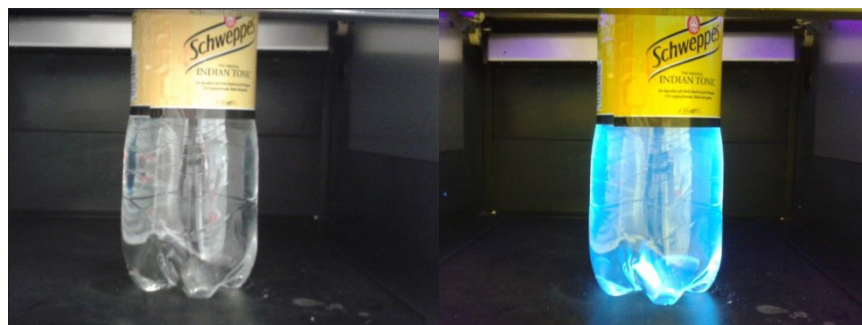
Figure 1. Tonic water illuminated with visible light (left) and a UV lamp (right). The glowing blue colour is due to the fluorescence of quinine.
