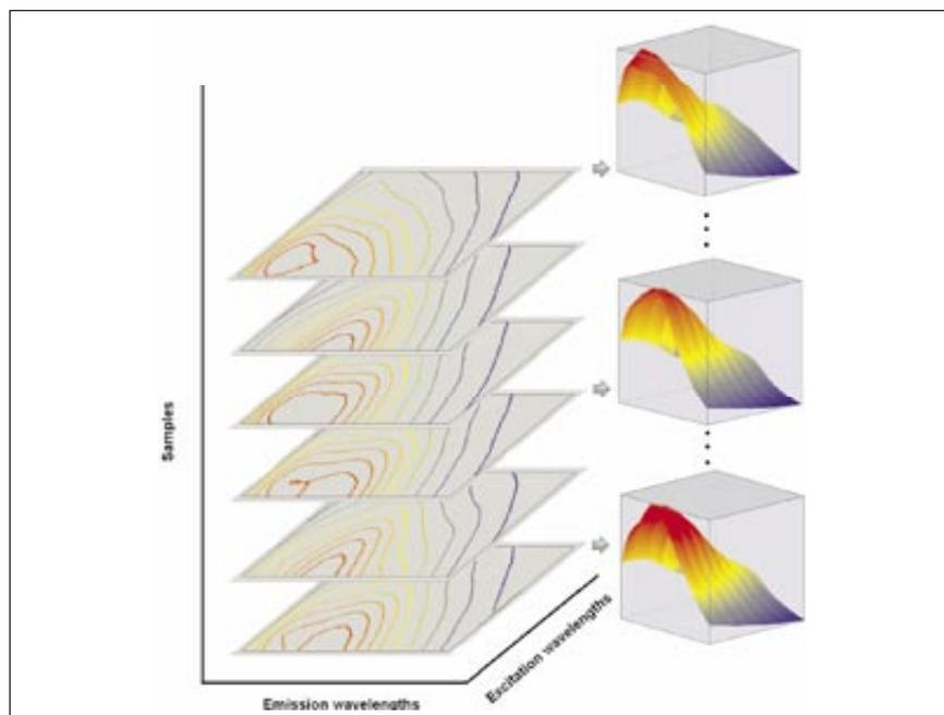
**Figure 6.** Six ex/em scans shown as contour plots of test samples containing Fluorescein, Eosin Y, Rhodamine 6G and Rhodamine B. Three are also shown as 2D-surface plots. The emission spectra were scanned between 500 and 600 nm using 460, 465, 470, 475, 480, 485, 490 and 495 nm excitations.
