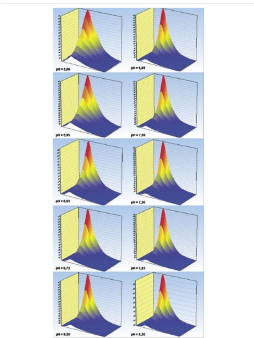
**Figure 4.** Emission spectra of fluorescein at pH=5.66, 5.95, 6.51, 6.72, 6.80, 6.88, 7.08, 7.36, 7.82 and 8.30 measured between 470 and 650nm using 390, 400, 410, 420, 430, 440, 450 and 460nm excitation.
