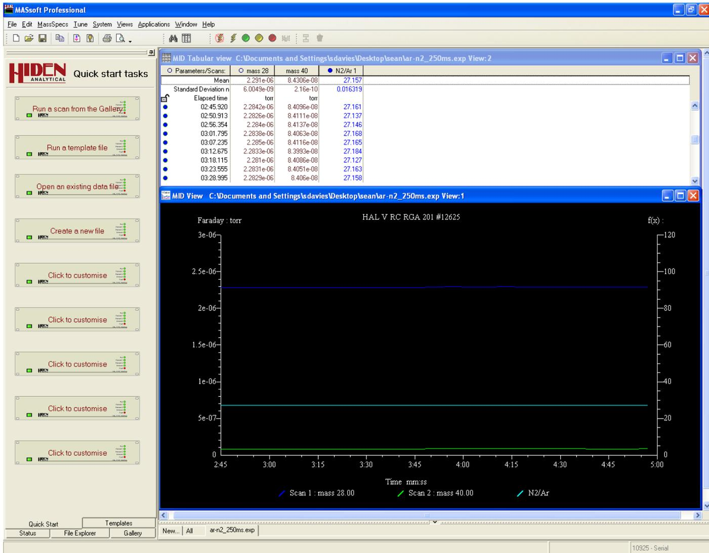
**Figure 2. MASsoft Professional tabular and graphical output data from HPR-40: N<sub>2</sub>, Ar and N<sub>2</sub>/Ar precision from MIMS sampled water**
