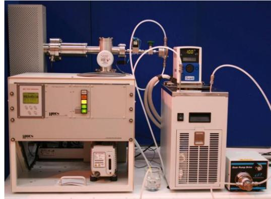
**Figure 1: HPR-40 (MIMS analysis of high precision  $N_2/Ar$  ratios for denitrification processes in marine and aquatic biology (shown with chiller system in line)**
