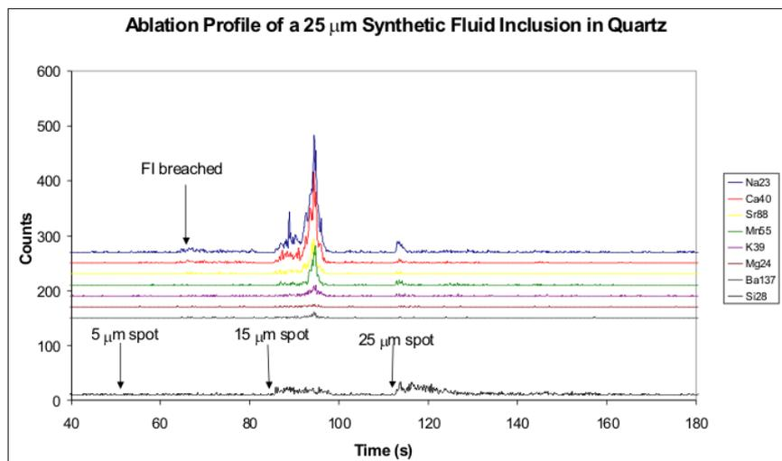
**Figure 2.** ICP-MS signal from ablation of a synthetic fluid inclusion, c. 25  $\mu\text{m}$  in diameter. In this example the inclusion was first breached using a very small (5  $\mu\text{m}$ ) laser spot, but there was no significant signal until it was fully opened with a 15  $\mu\text{m}$  laser spot. This ablation removed the bulk of the contents, although the signal is irregular, and further ablation with a 25  $\mu\text{m}$  spot removed a small amount of additional salts.
