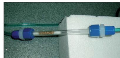
**Figure 5.** Gold trap attached in-line to carrier gas line to scrub Hg.
