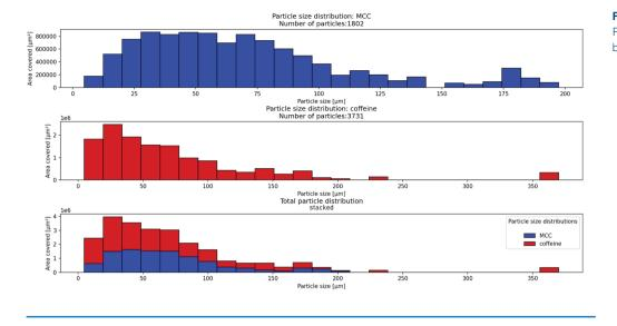
Fig. 4 Particle statistics received by the tablet analyzer.
