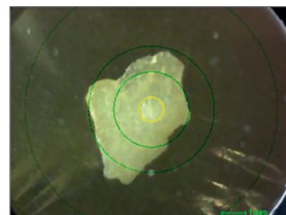
Figure 4. Photograph of contaminant (the yellow circle is the x-ray irradiation range: 1 mm Ø).
