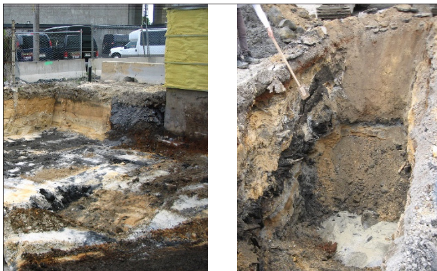
Typical test pits in geo-environmental engineering site soil characterisation. One attribute rules the day: “significant heterogeneity”. It is obvious that any single field sample (a grab sample in the TOS parlance) will not be able to represent the entire site. For this job, diligent compliance with the TOS’ principle of composite sampling is necessary (see part 2).
