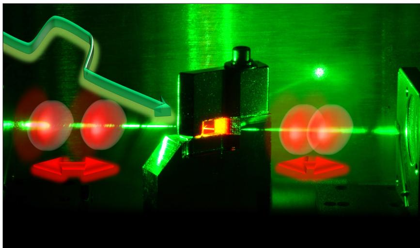
Light pulses can form pairs in ultra-short pulse lasers. The pulse intervals (red) can be precisely adjusted by making certain changes to pump beam (green). Image: UBT.
