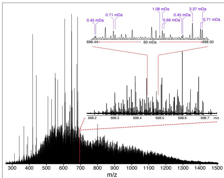
**Figure 3.** Stitched mass spectrum of the non-distillable fraction of a heavy crude oil, with peaks spanning  $m/z$  260–1505. The spectrum was obtained by stitching 65 windows, each with an  $m/z$  width of 24, with steadily increasing acquisition time per segment to result in near constant resolving power across the  $m/z$  range. An enlarged region, showing assignments for  $m/z$  698, is shown. Reproduced from Reference 3 under a Creative Commons Attribution licence.
