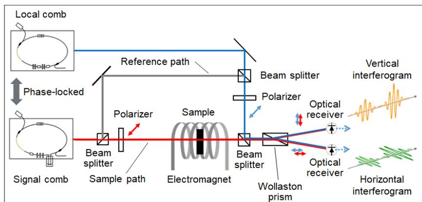
Block diagram of Faraday effect measurement system using dual-comb spectroscopy. The signal comb (red line) passes through the sample and is superposed with the local comb (blue line). The vertical and horizontal components of the interference signal are detected by the two optical receivers. Applying magnetic field to the sample, the Faraday effect (Faraday rotation angle) is measured. Credit: ©The University of Electro-Communications, Kaoru Minoshima and NEOARK.
