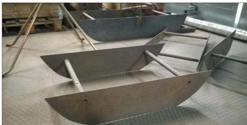
**Figure 2.** Example of a “stopped belt” sampling frame allowing a complete cross-section of the ore stream to be extracted. This will serve as a reference to the online sampling system (Figure 1). Image credit: LKAB.
