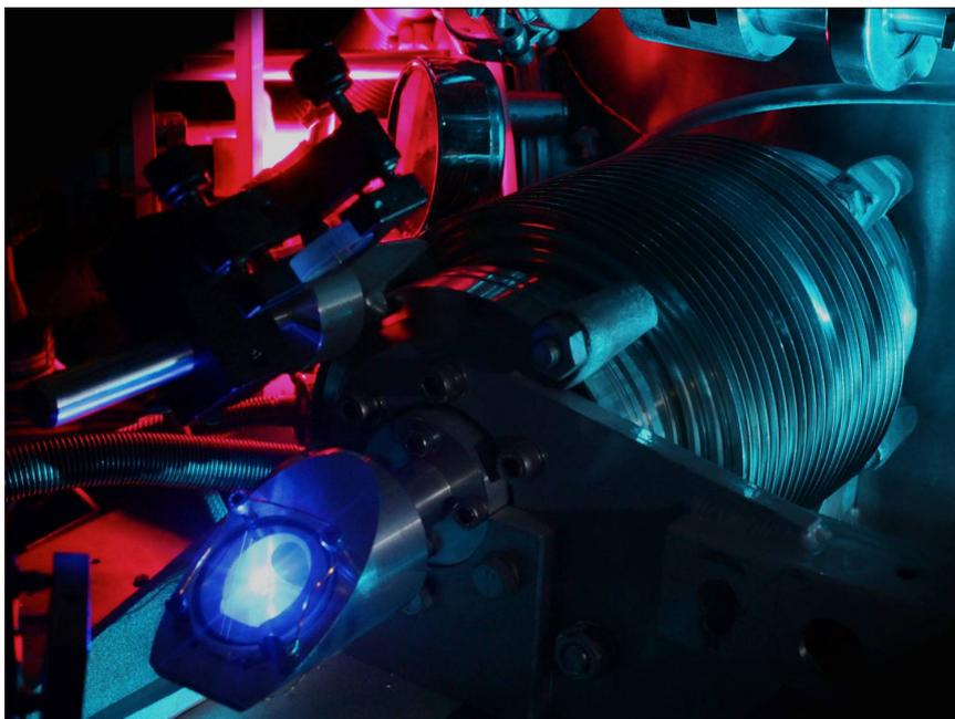
This photo shows the vacuum chamber used to measure the  $2S-4P$  transition frequency in atomic hydrogen. The purple glow in the back stems from the microwave discharge that dissociates hydrogen molecules into hydrogen atoms. The blue light in the front is fluorescence from the ultraviolet laser that excites the atoms to the  $2S$  state. The turquoise blue glow is stray light from the laser system used to measure the frequency of the  $2S-4P$  transition. (Photo: MPQ)
