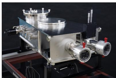
Imaging comes to certain McPherson VUV spectrometers.
