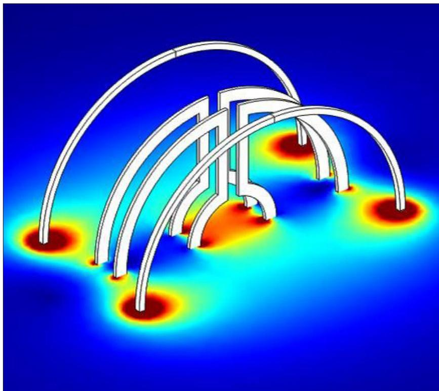
Two Lenz lenses are arranged in a Helmholtz coil pair. Simulation shows how the Lenz lenses focus magnetic flux. (Illustration: Nils Spengler/KIT)
