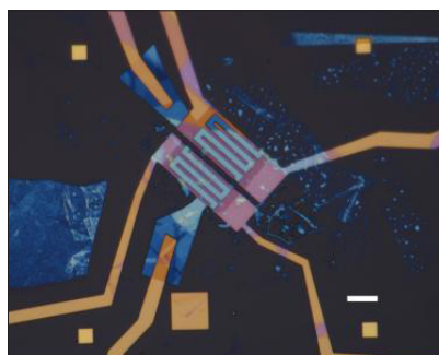
An optical micrograph of two typical on-chip spectrometers. Scale bar: 8 \mu\text{m}
