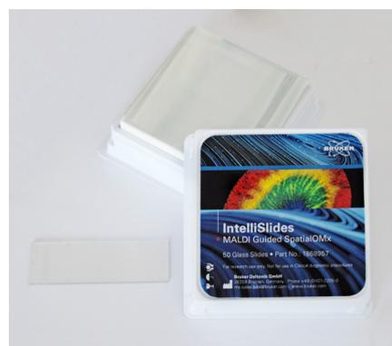
tive surface to indicate where to place the tissue sample, a bar code and tracking number. IntelliSlides automation removes sources of inefficiency from sample loading, as they are inherently correctly labelled, oriented properly and MALDI image registration occurs at the touch of a button.
