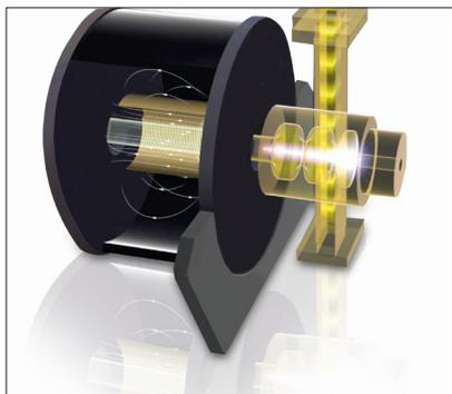
The FLUTE linear accelerator accelerates electron clouds in order to generate terahertz rays. (Illustration: KIT)
