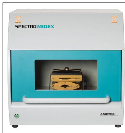
The Spectro Midex MID05 ED XRF spectrometer for precious metals.
