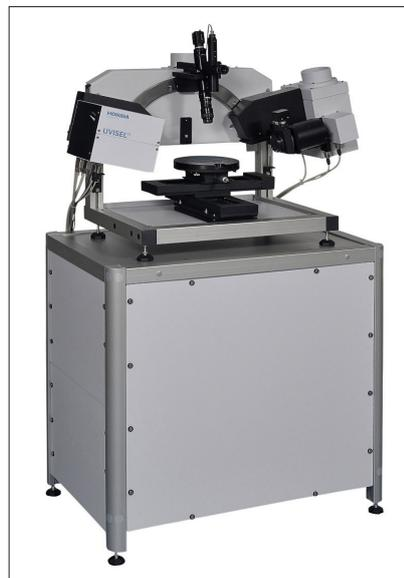
Horiba Scientific's Uvisel Plus, a modular ellipsometer for thin film samples.
