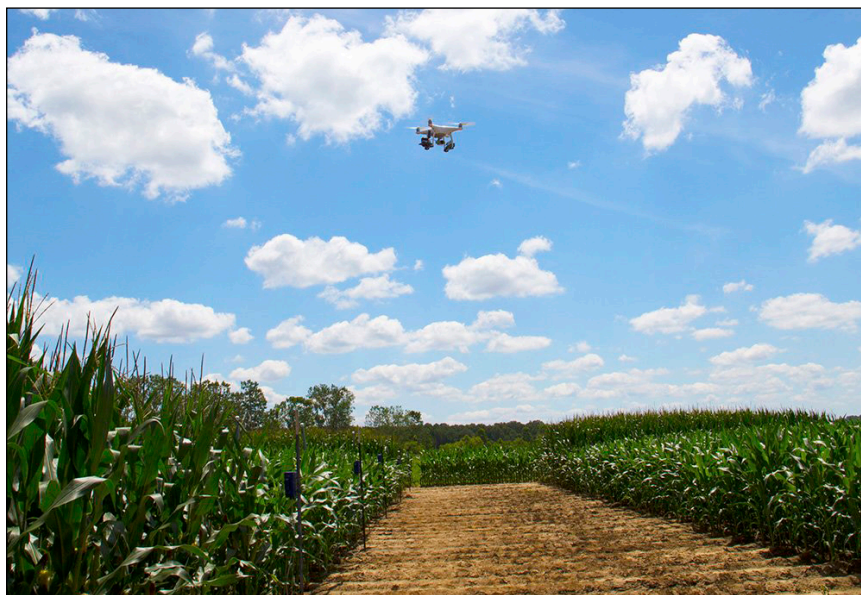
A standard RGB camera attached to a drone, combined with AI deep learning, can provide crop health colour maps, a new study shows. Photo: Diane Godwi
