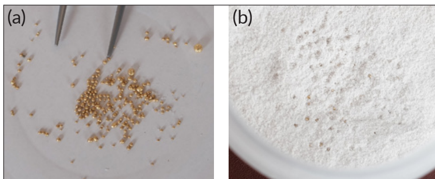
Figure 2. a) Approximately 300 gold grains, ranging in size from 100 μm to 300 μm, and b) finely ground quartz matrix showing gold grains on surface before mixing. Illustration copyright: RCAM teaching collection; used with permission.
