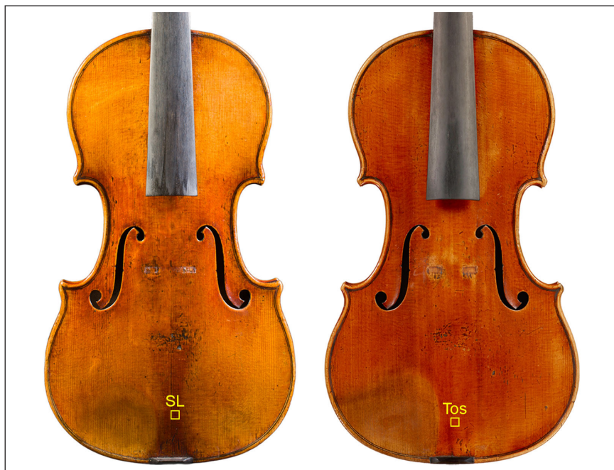
A nanometre-scale imaging technique has revealed a protein-based layer between the wood and the varnish coating of these two Stradivarius violins. Credit: Adapted from Analytical Chemistry , doi: 10.1021/acs.analchem.2c02965
