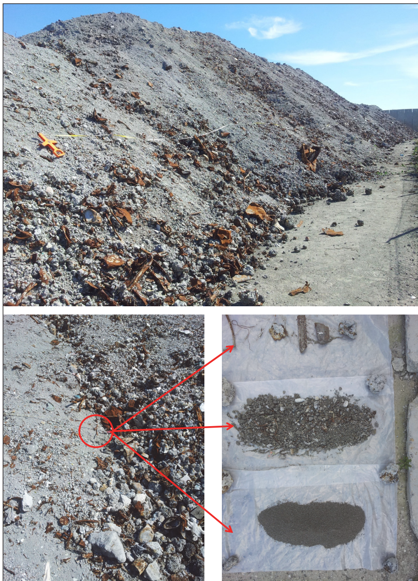
Figure 4. How to arrive at a reliable analytical result for a much more complex lot, e.g. incinerator bottom ash. A simple food processor comminution is not enough, much more powerful crushing technologies are needed, as well as another analytical technique (XRF), but the necessary separation into size-classes is identical to what is needed also for a bag of chips, even though the primary sampling step is clearly also critical. Photo credits: Center for Minerals and Materials (MIMA), GEUS ( https://www.geus.dk ).
